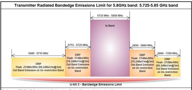
Refer as FCC KDB 789033 D02 v01, G)2)c)(i) specifying that if a non-restricted-band out-of-band emission satisfies both the average and peak limits of 15.209, it is not required to satisfy the -27 dBm or -17 dBm peak emission limit. Reason for change: to ensure that emission requirements in the non-restricted bands are not more stringent than those in the restricted bands.
