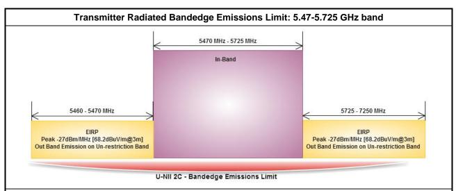
Refer as FCC KDB 789033 D02 v01, G)2)c)(i) specifying that if a non-restricted-band out-of-band emission satisfies both the average and peak limits of 15.209, it is not required to satisfy the -27 dBm or -17 dBm peak emission limit. Reason for change: to ensure that emission requirements in the non-restricted bands are not more stringent than those in the restricted bands.
