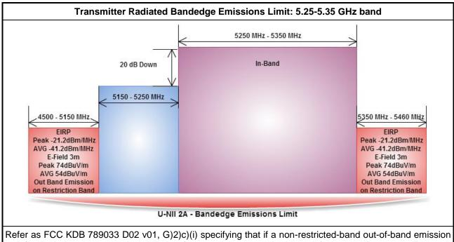
Refer as FCC KDB 789033 D02 v01, G)2)c)(i) specifying that if a non-restricted-band out-of-band emission satisfies both the average and peak limits of 15.209, it is not required to satisfy the -27 dBm or -17 dBm peak emission limit. Reason for change: to ensure that emission requirements in the non-restricted bands are not more stringent than those in the restricted bands.
