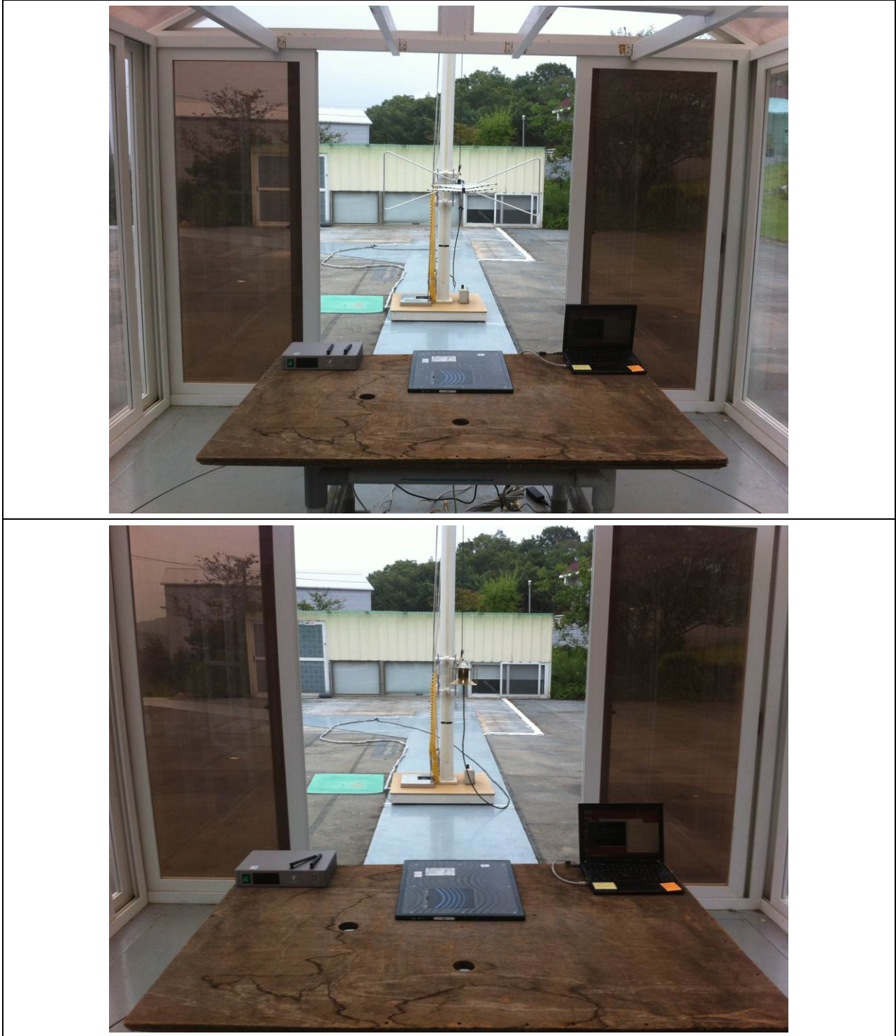
Figure.1. Radiated Emission Test Setup
