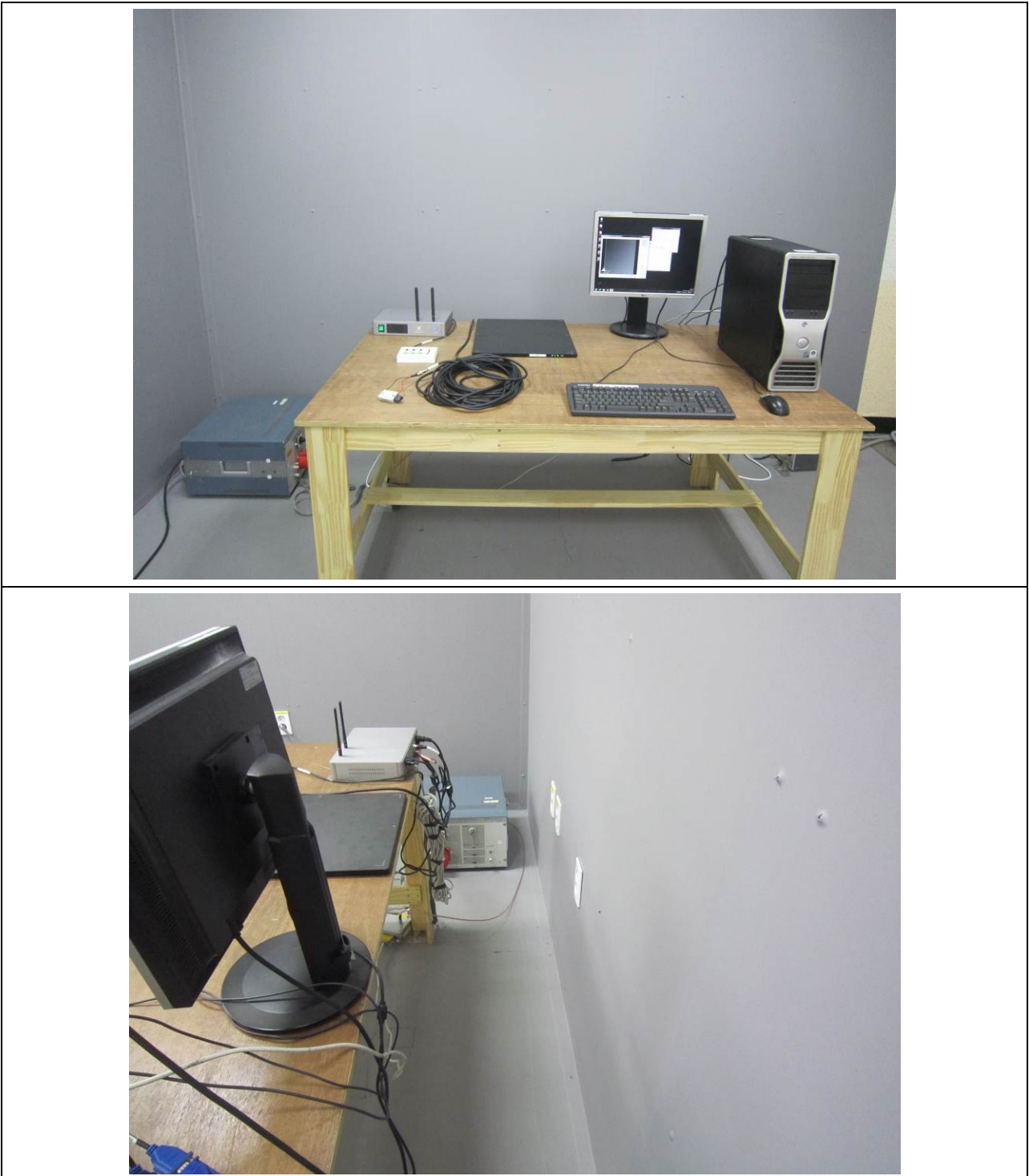
Figure.2. Test Setup for Conducted Emissions
