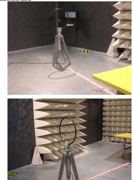
2 Photographs of Radiated Emissions Test Configuration For radiated emissions 9kHz~30MHz
