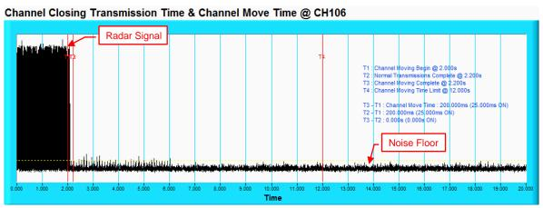
**NOTE:** T1 denotes the start of Channel Move Time upon the end of the last Radar burst. T2 denotes the data transmission time of 200ms from T1. T4 denotes the 10 second from T1 to observe the aggregate duration of transmissions.
