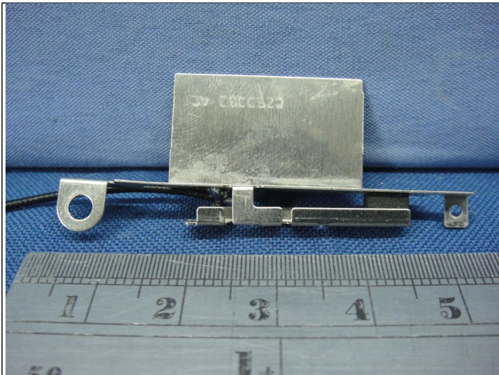
Antenna (Brand : WNC, Model : 81-EBJ15.005<3.62dBi>)
