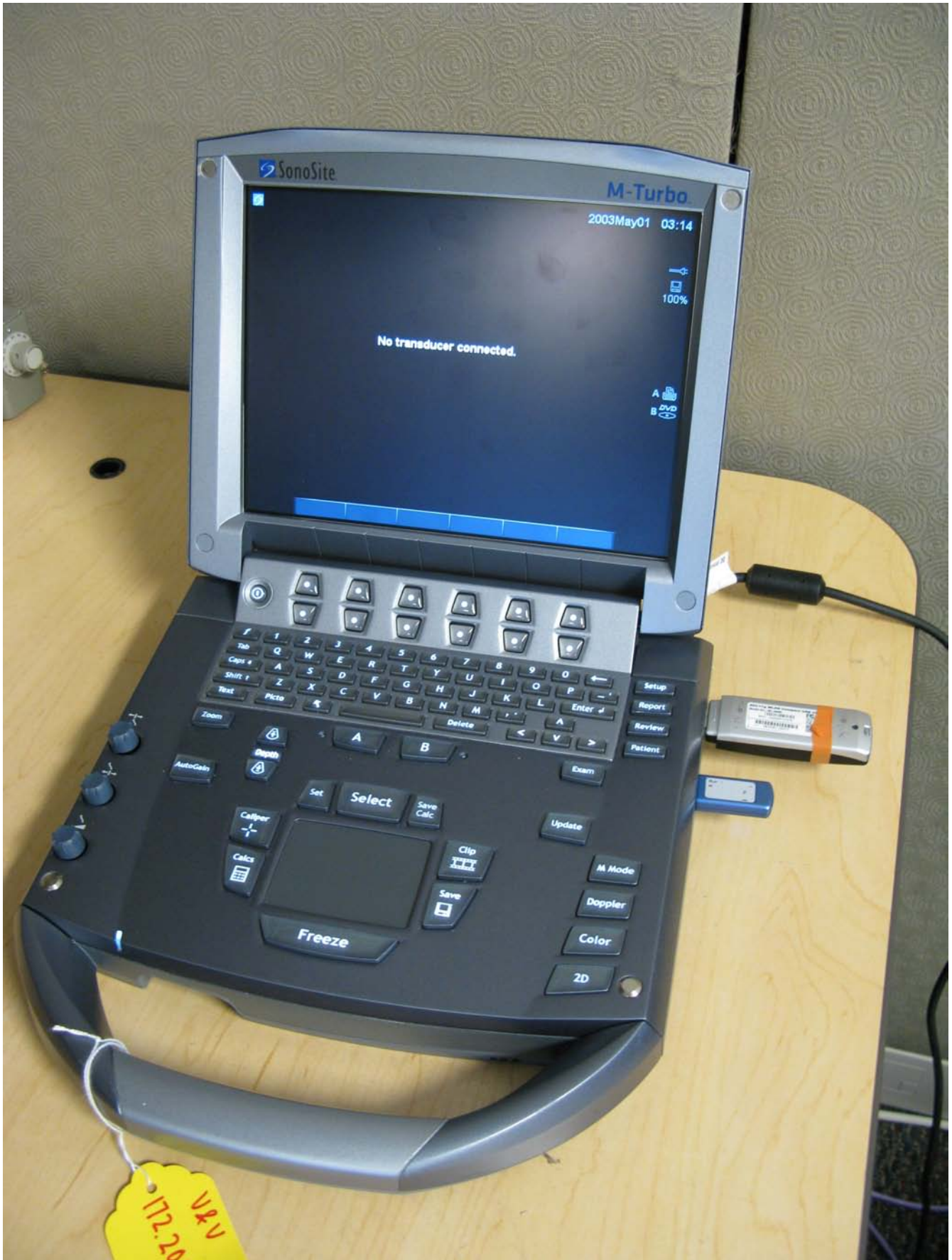
Illustration 1: M-Turbo unit with Bluetooth and 802.11 Dongles inserted
