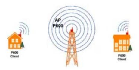
Wireless Bridge: This mode allows the connection of one or more remote LANs with a central LAN.
