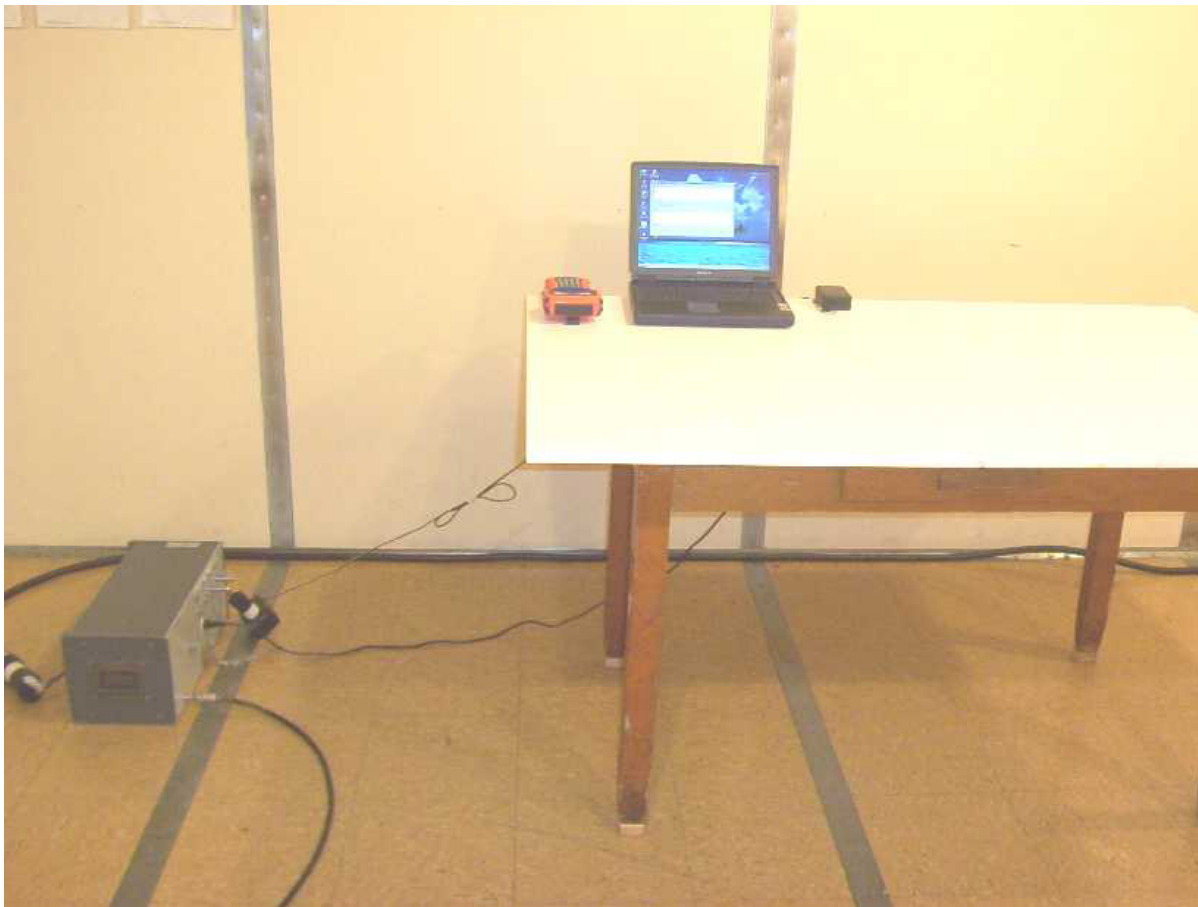
Photo 1: Conducted Emission Test Setup, JETT.XL – Front View
