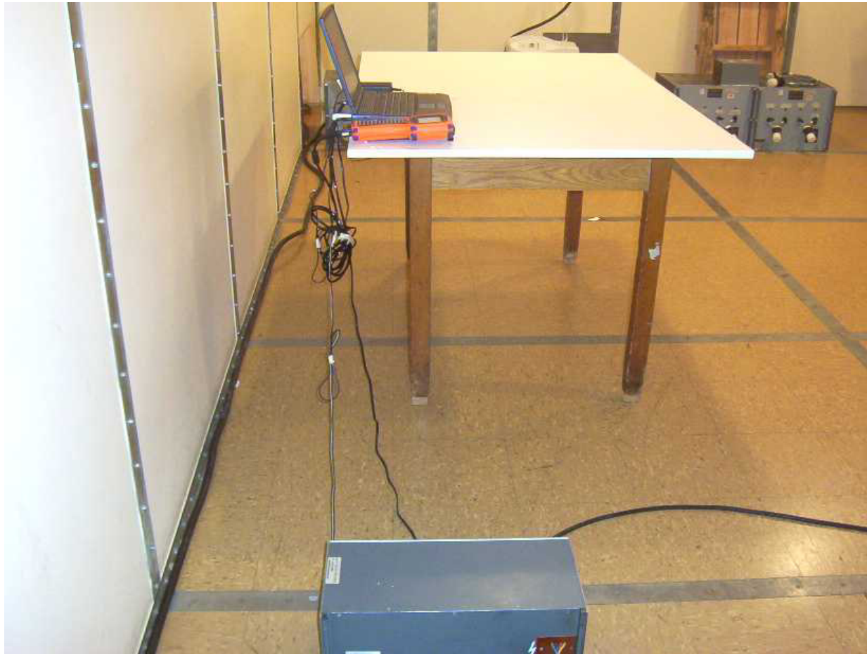
Photo 2: Conducted Emission Test Setup, JETT.XL – Side View
