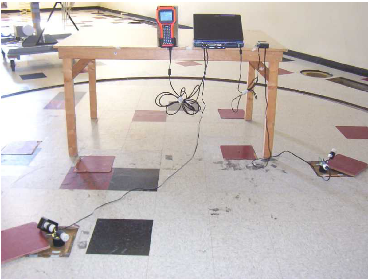
Photo 1: Radiated Emission Test Setup – Vertical Orientation, Front View
