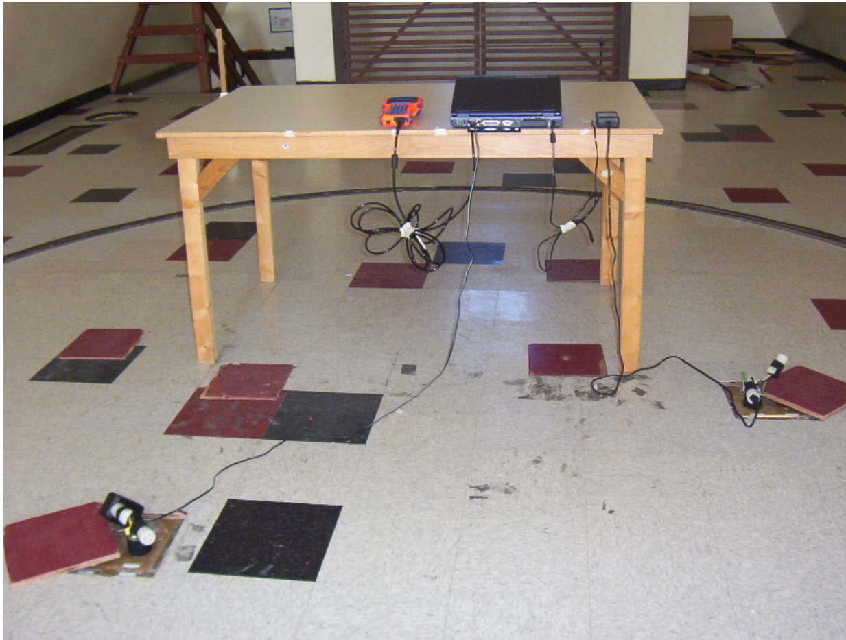
Photo 5: Radiated Emission Test Setup – Flat Orientation, Front View
