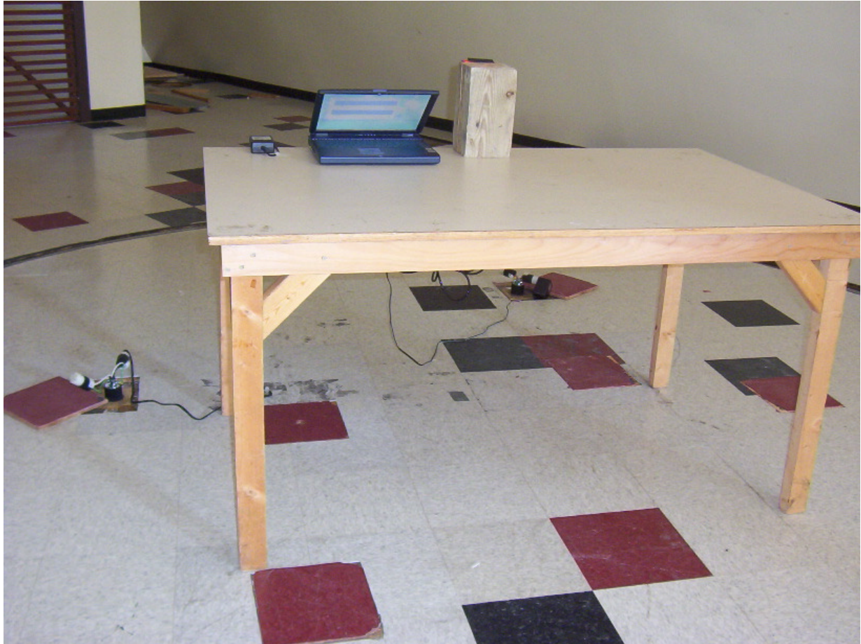
Photo 2: Radiated Emission Test Setup – Vertical Orientation, Rear View
