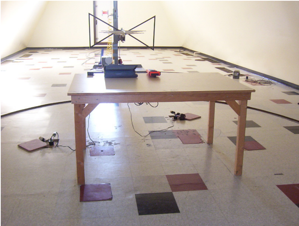
Photo 6: Radiated Emission Test Setup – Flat Orientation, Rear View
