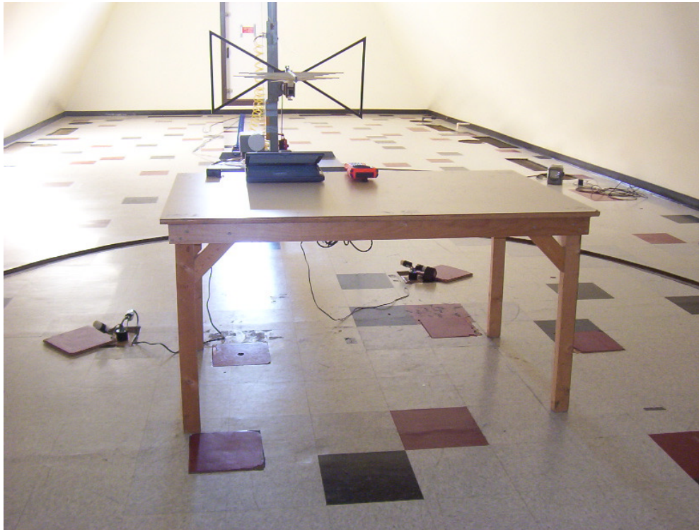
Photo 9: Radiated Emission Test Setup – Flat Orientation, Rear View
