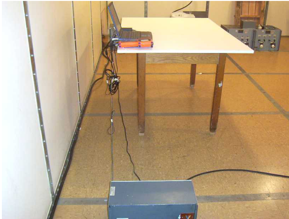
Photo 11: Conducted Emission Test Setup, JETT.XL – Side View
