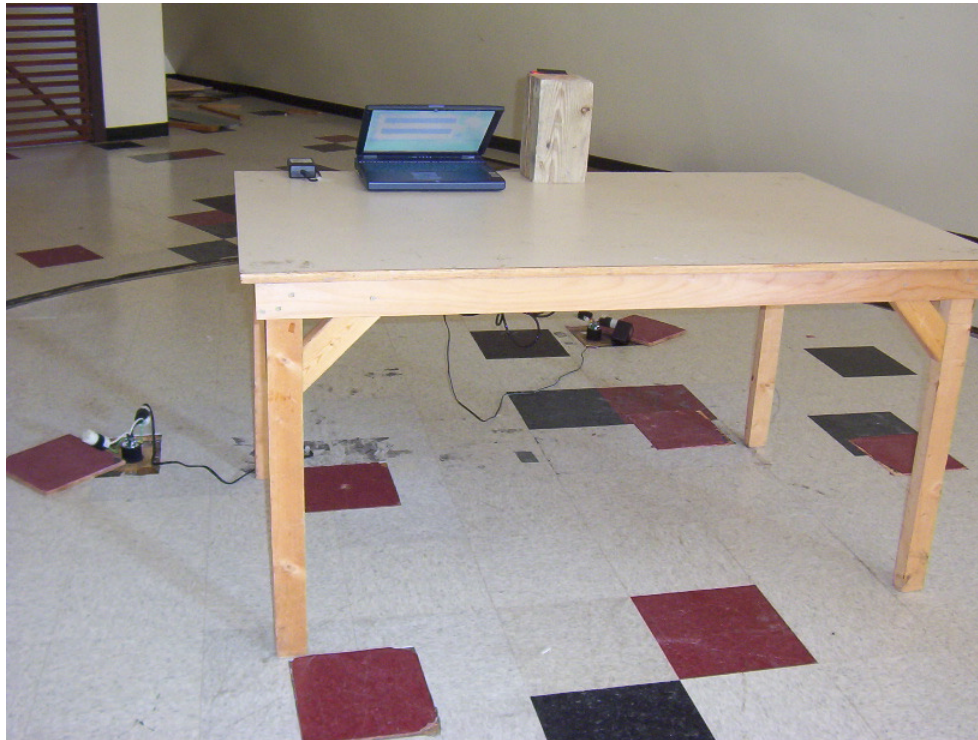
Photo 5: Radiated Emission Test Setup – Vertical Orientation, Rear View
