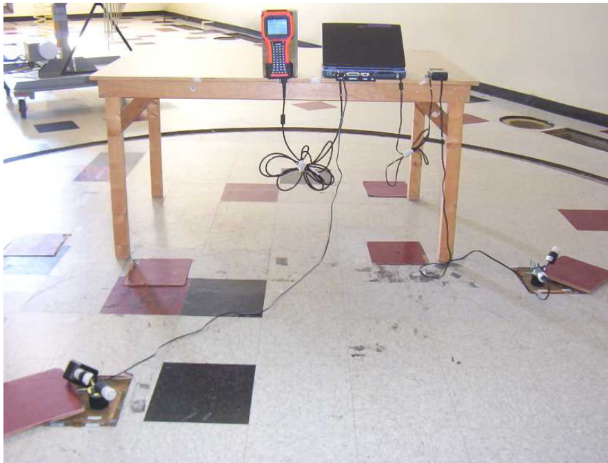
Photo 4: Radiated Emission Test Setup – Vertical Orientation, Front View
