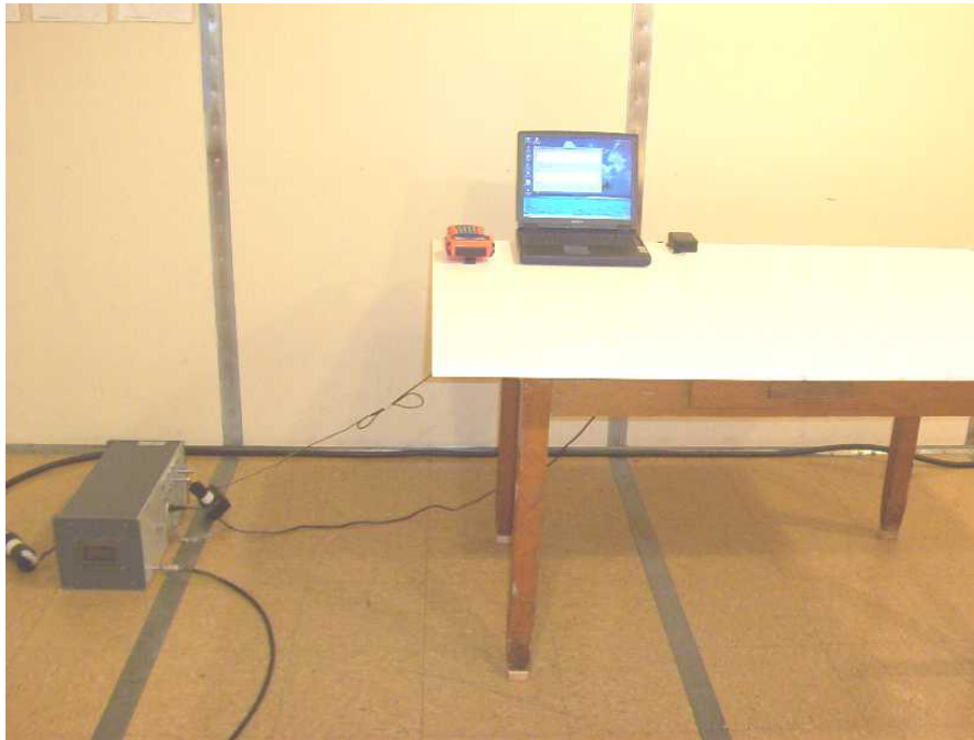
Photo 10: Conducted Emission Test Setup, JETT.XL – Front View
