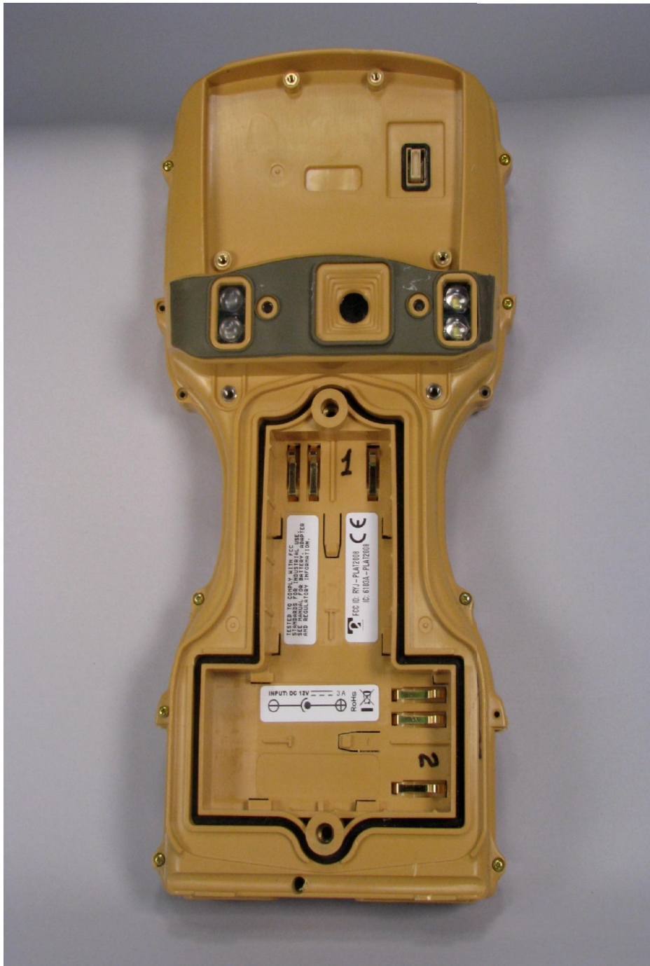
REAR OF PLAT2008 WITH BATTERY COMPARTMENT COVER, BATTERY REMOVED SHOWING LABEL PLACEMENT
