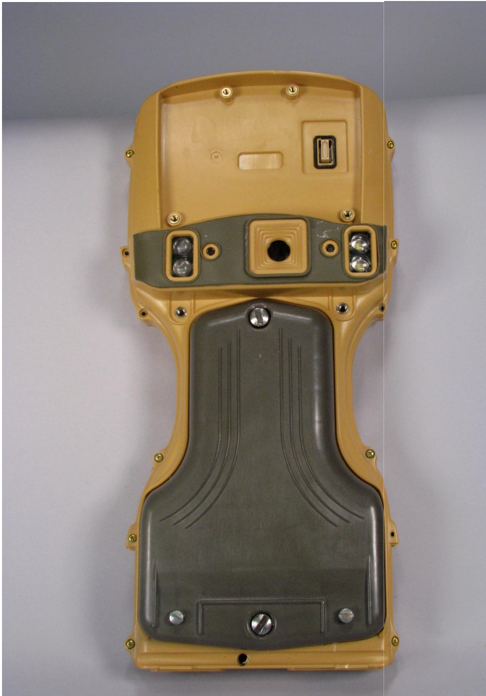
REAR OF PLAT2008 ENCLOSURE WITH BATTERY COMPARTMENT COVER IN PLACE. CAMERA LENS, 4 WHITE LEDs, OPENINGS FOR 2 RED LASER DIODES AND CONNECTOR FOR OPTIONAL PACK VISIBLE.
