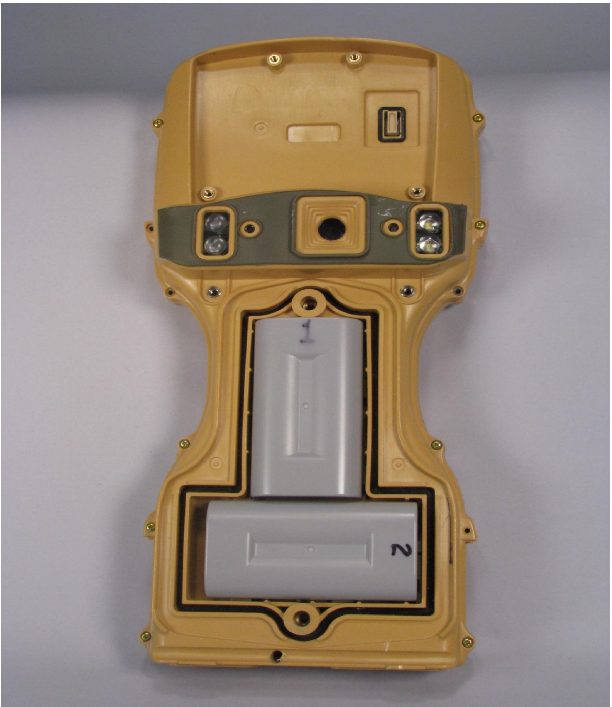
REAR OF PLAT2008 WITH BATTERY COMPARTMENT COVER REMOVED. BATTERIES IN PLACE
