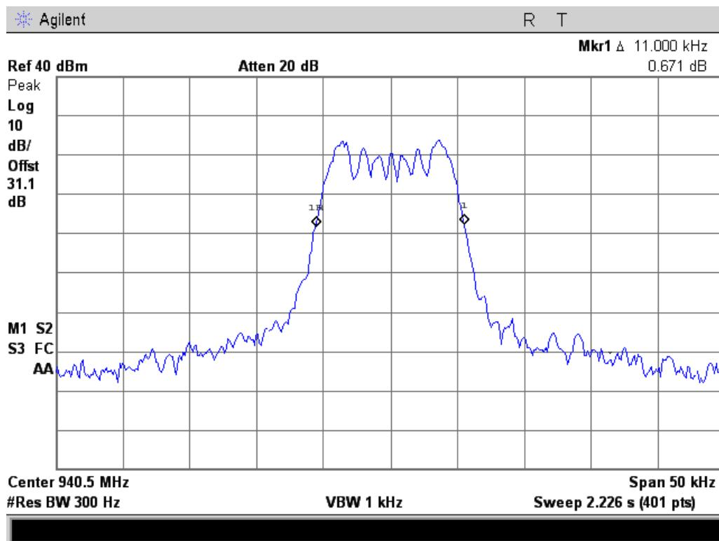
The occupied bandwidth of both operational bands was similar in shape and bandwidth to the input signal.
