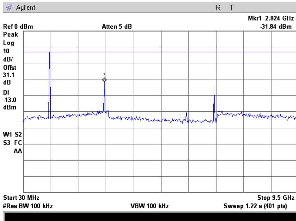
Only harmonic products of the fundamental signal are detectable. There are no intermodulation products.
