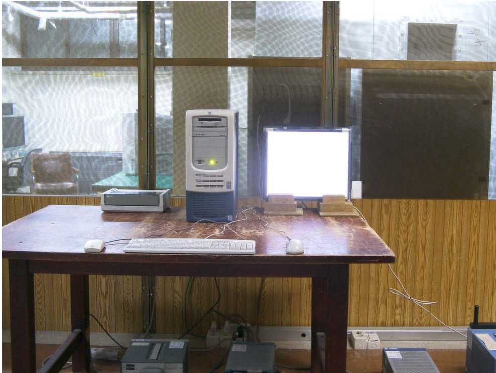
Conducted Emissions - Front View
