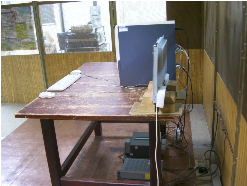
Conducted Emissions - Front View
