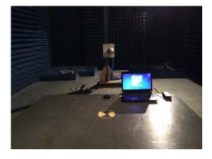
3. Photos of Conduction Emission Test
