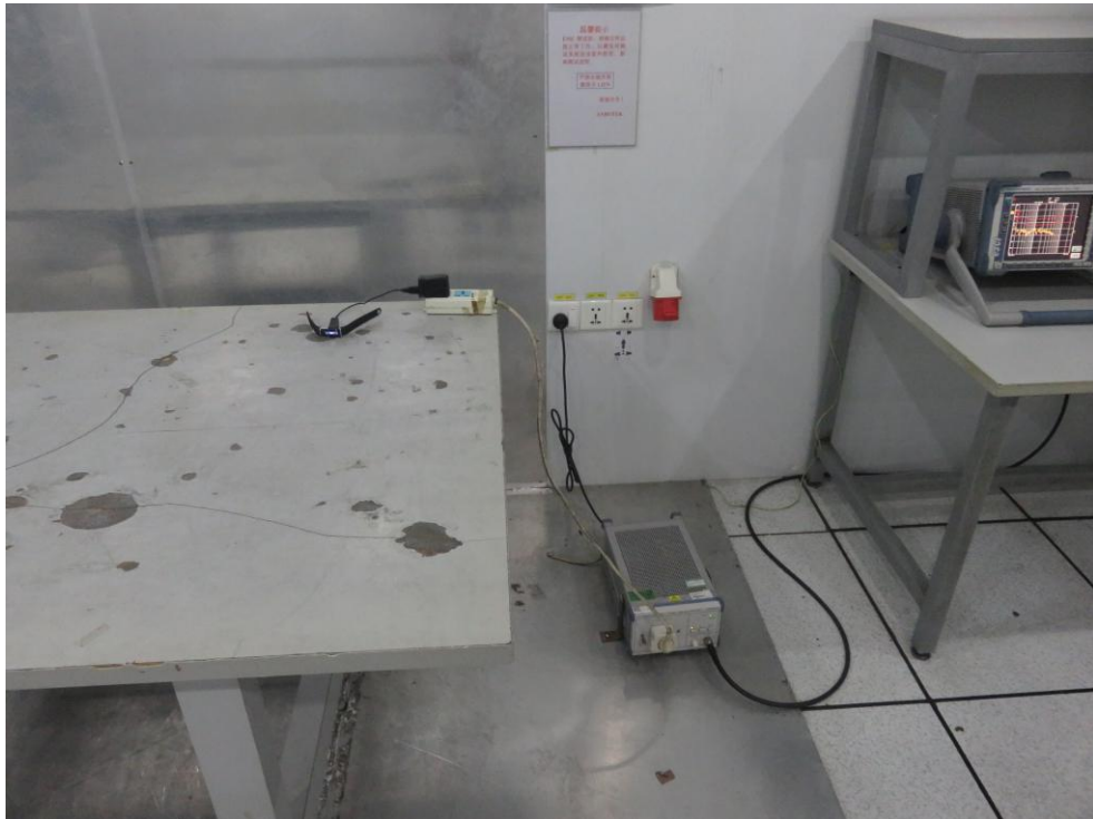
Photo of Conducted Emission Measurement
