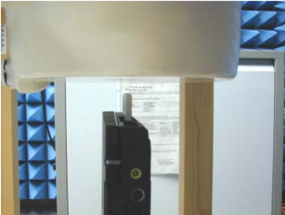
Fig.7 Edge of the PC at 90° and at a distance of 1.5 cm from the base of the phantom.
