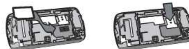
3. Insert the battery (with the connectors facing the connectors of the phone) and press until it clips.
