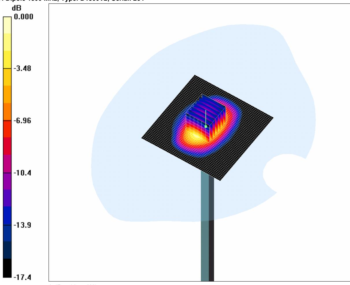
Communication System: CW; Frequency: 1800 MHz; Duty Cycle: 1:1
