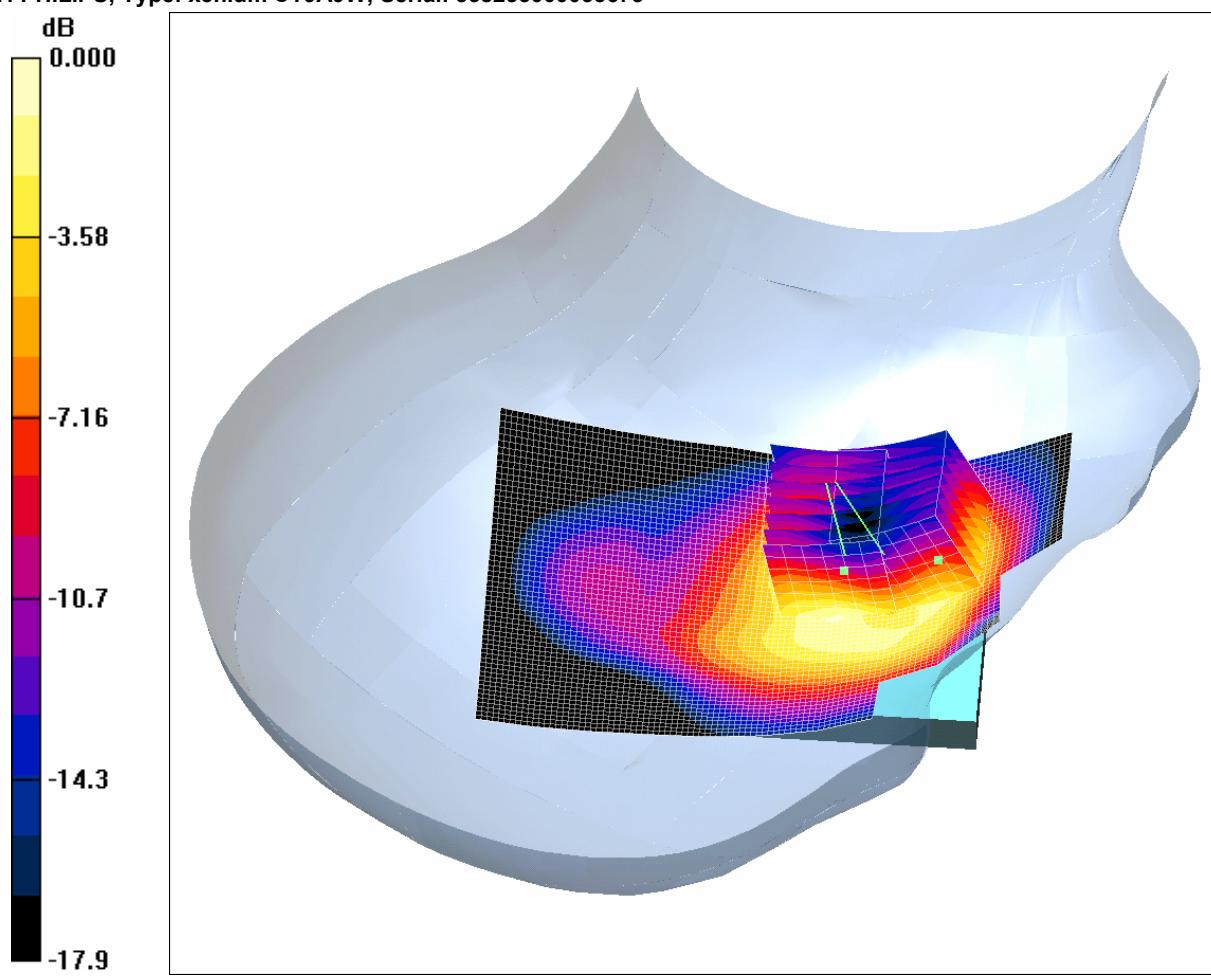
Communication System: PCS 1900; Frequency: 1850.2 MHz; Duty Cycle: 1:8.3
