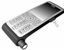
*To remove the micro SD card, push down the card into its slot and release it. The card will spring out of the slot.*
