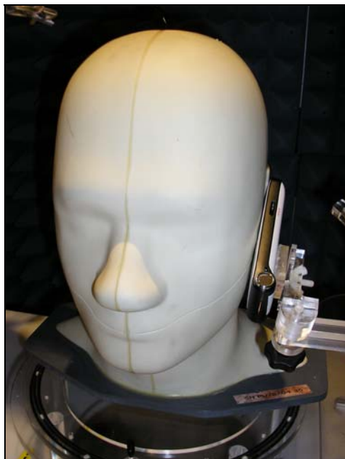
Figure 33: Positional Photograph of the CT9A9j Handset in LH Cheek Position.
