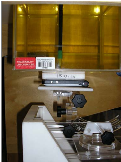
Figure 37: Positional Photograph of the CT9A9j Handset in front facing Position. 15mm separation.
