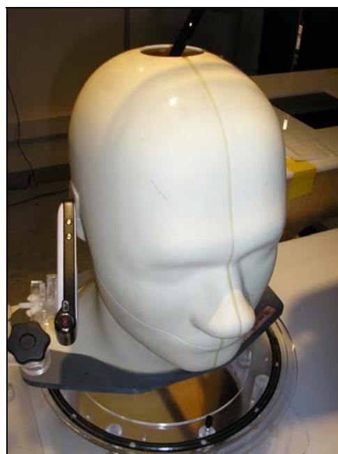
Figure 36: Positional Photograph of the CT9A9j Handset in RH 15° Position.
