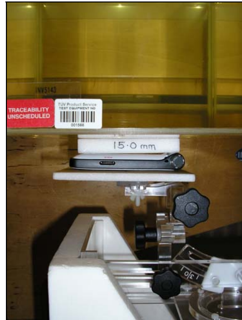
Figure 38: Positional Photograph of the CT9A9j Handset in rear facing Position 15mm separation.
