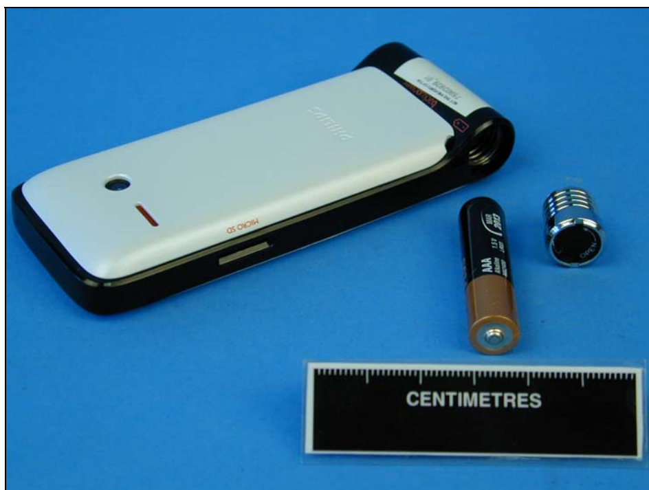
Figure 42: Rear View – Alkaline Battery Removed.
