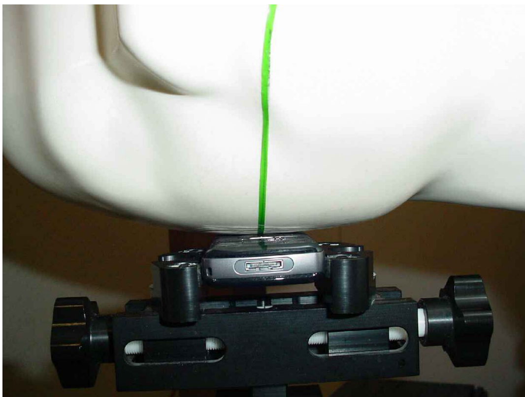
Photo 15: Test position right hand touched
