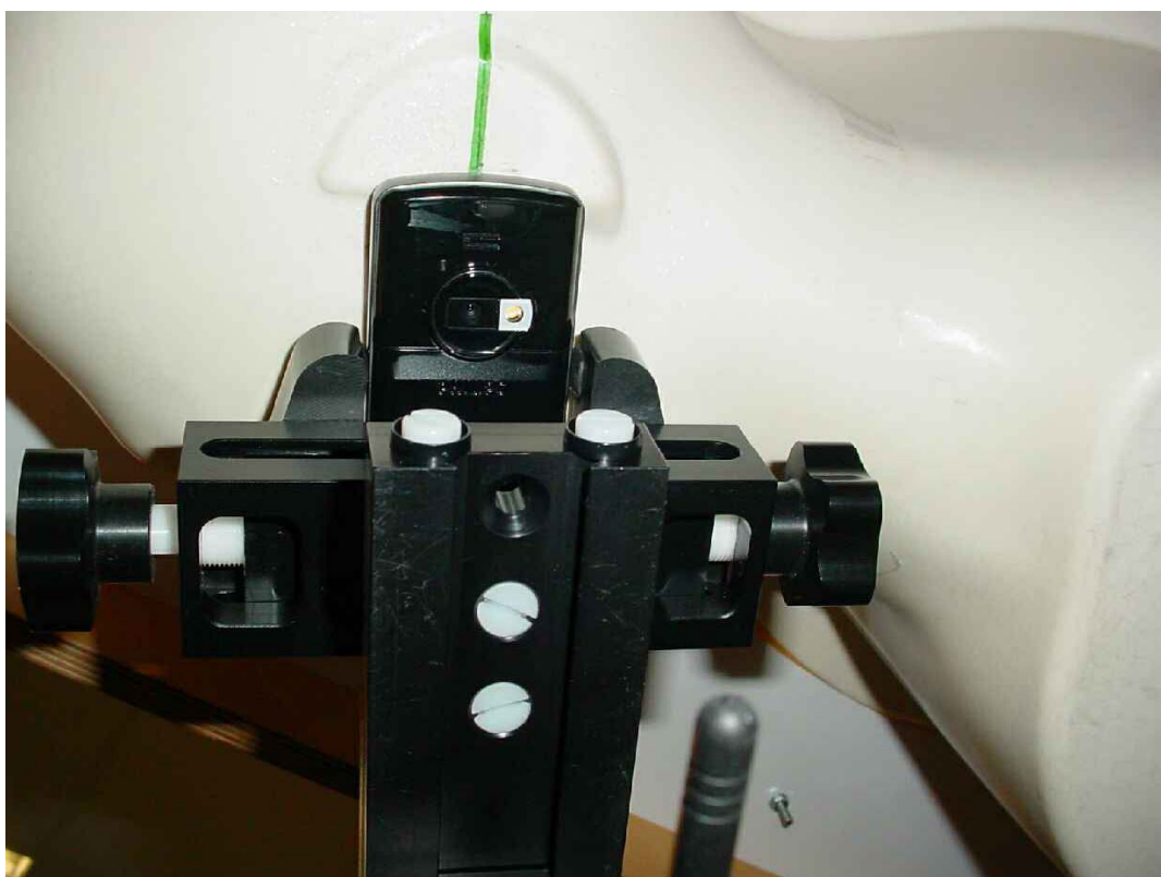
Photo 11: Test position left hand touched
