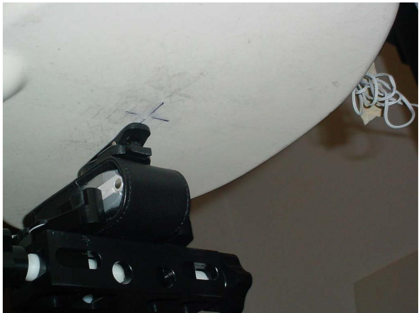
Using the Philips accessory the distance between antenna and phantom is around 28 mm
