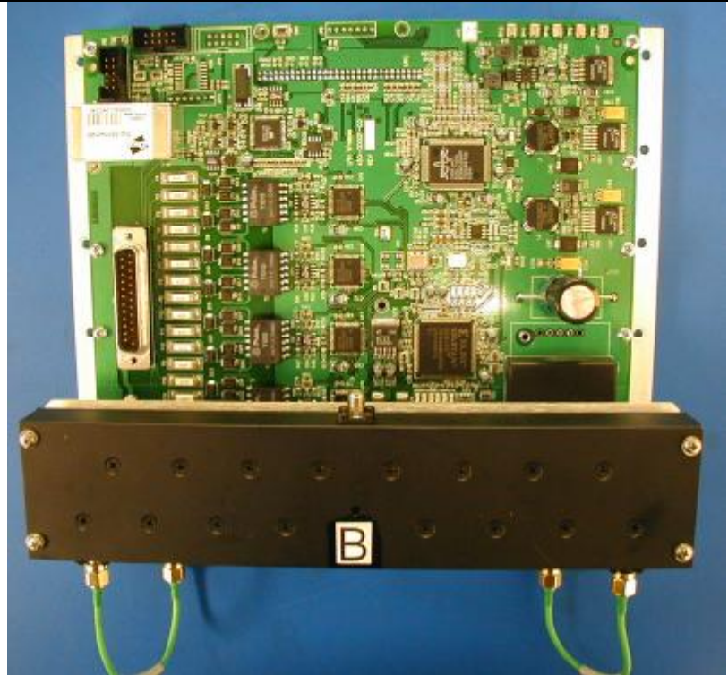
Figure 8-3 Electronics Package Removed From the ODU
