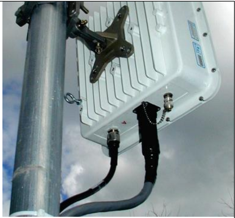
Figure 4-4 Typical ODU Mast Mount Mechanical Installation
