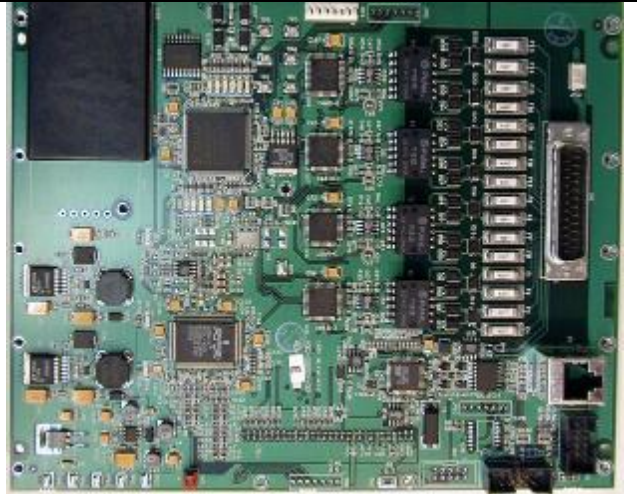
Figure 8-6 Electronics Package with Duplexer and Cover Removed
