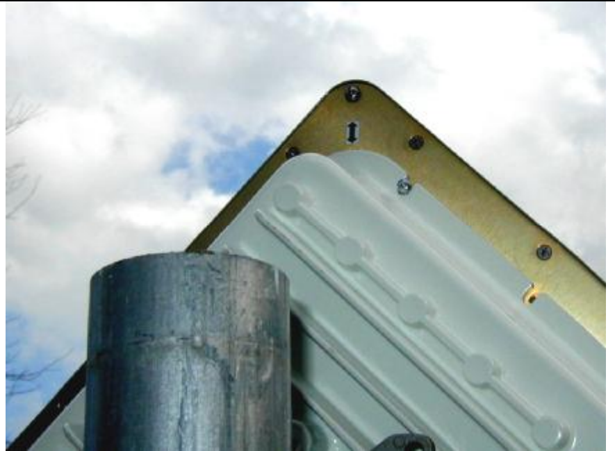
Figure 4-5 Integral Antenna Polarization Indication
