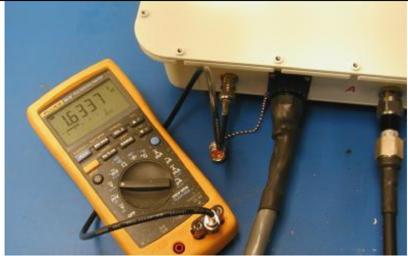
Figure 5-12 ODU RSSI Test Port
