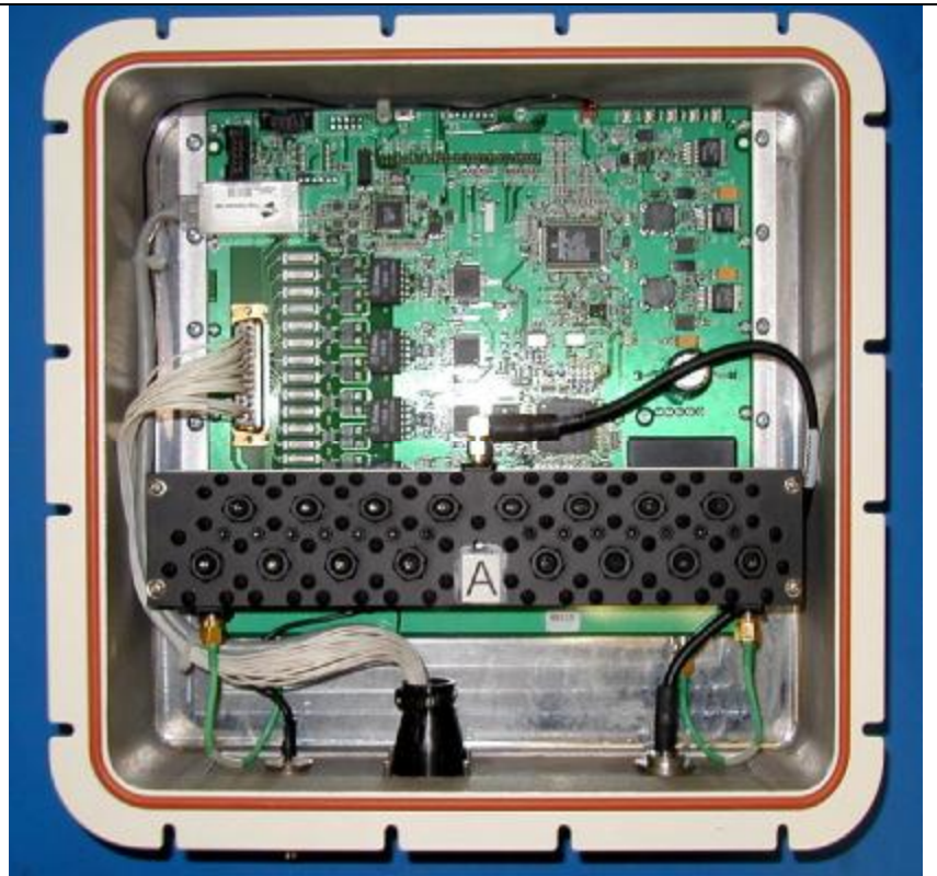
Figure 8-2 ODU with cover removed.
