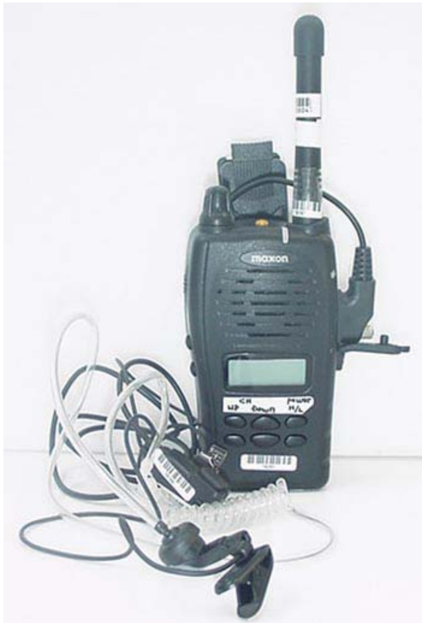
DUT with Earbud / Lapel-Microphone accessory
