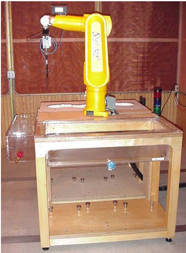
DASY4 SAR Measurement System with validation phantom
