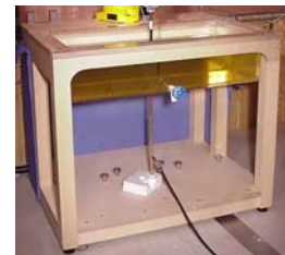
Validation Planar Phantom
