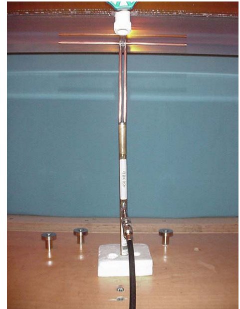
450MHz Dipole Setup
