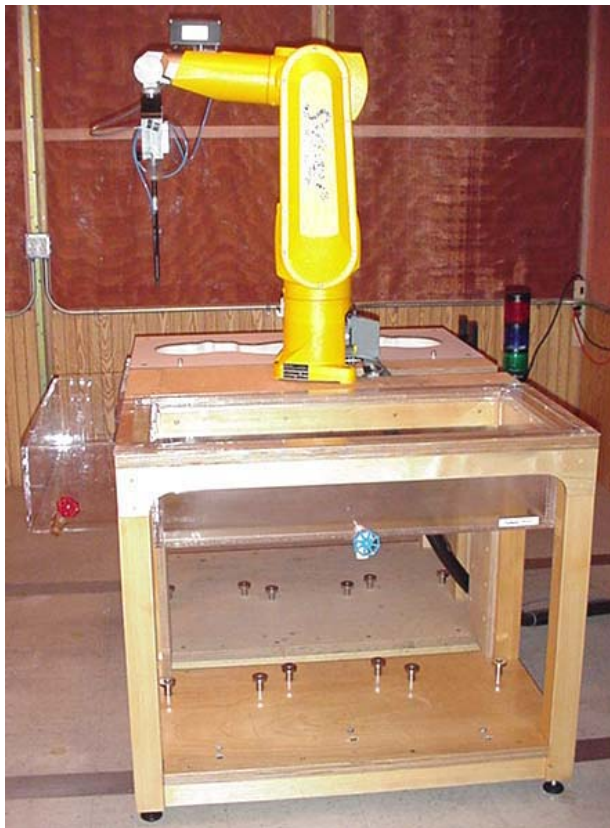
DASY4 SAR Measurement System with validation phantom
