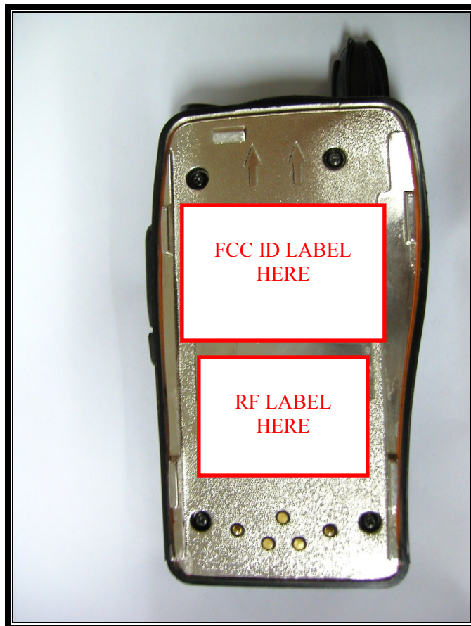
PHOTOGRAPH 1: FCC ID & RF LABEL LOCATIONS
