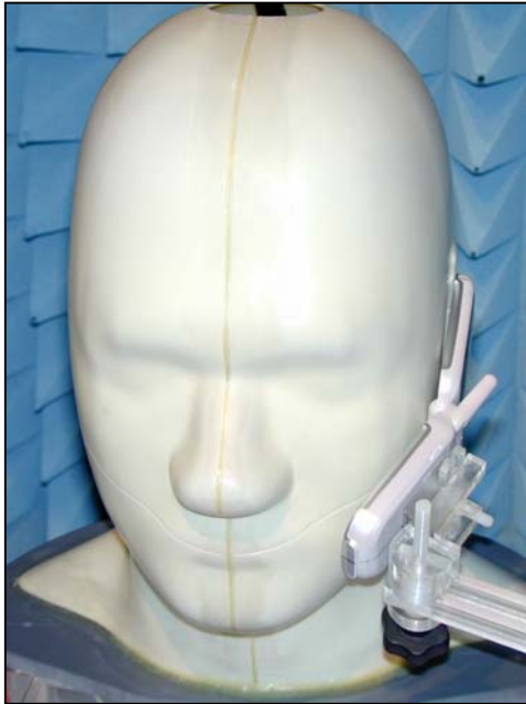
Figure 30. Positional photograph of the MX-V30 Handset in the Left-hand Cheek Position
