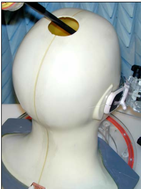
Figure 32. Positional photograph of MX-V30 Handset in the Right-hand Cheek Position
