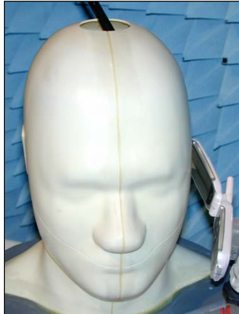
Figure 31. Positional photograph of MX-V30 Handset in the Left-hand 15 Degree Position
