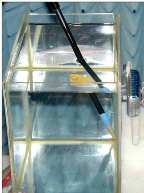
Figure 32. A Positional photograph of the MX-C99 Handset Fitted with Normal Battery positioned Rear Facing 10mm from the Flat Phantom.
