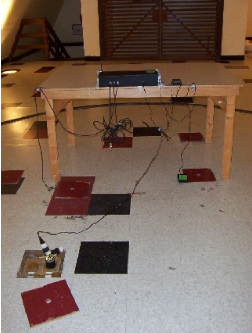
Photo 2: Radiated Emission Test Setup – Rear View
