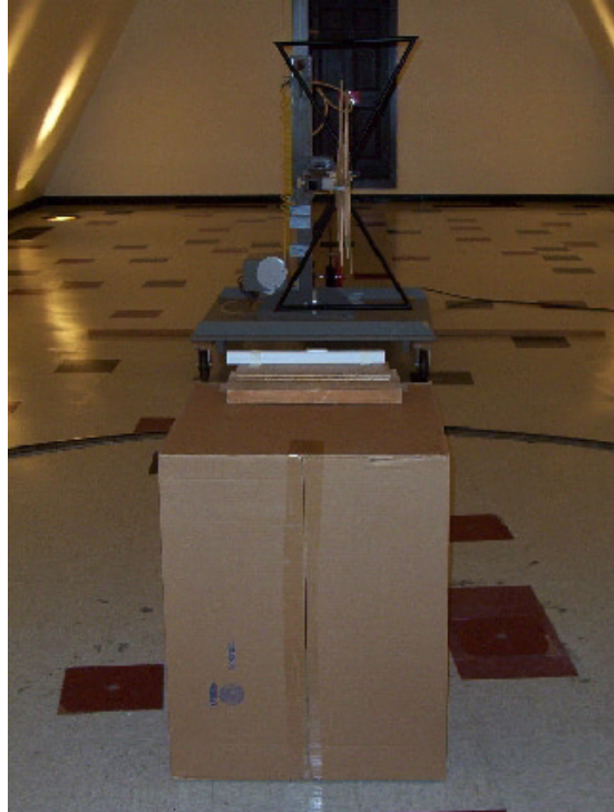
Radiated Emission Test Setup – EUT on Side, Tx Light Facing Up
