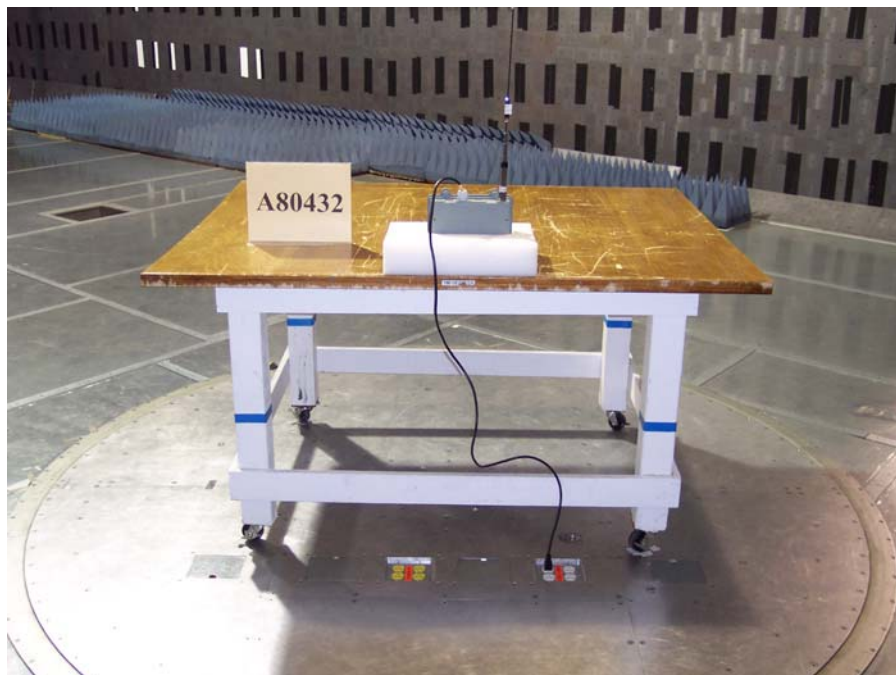
Figure 2. Representative Test Setup – Radiated Emissions.
