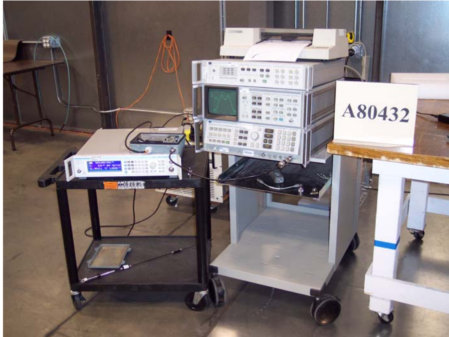
Figure 3. Representative Test Setup – Conducted Emissions, Antenna Terminals.
