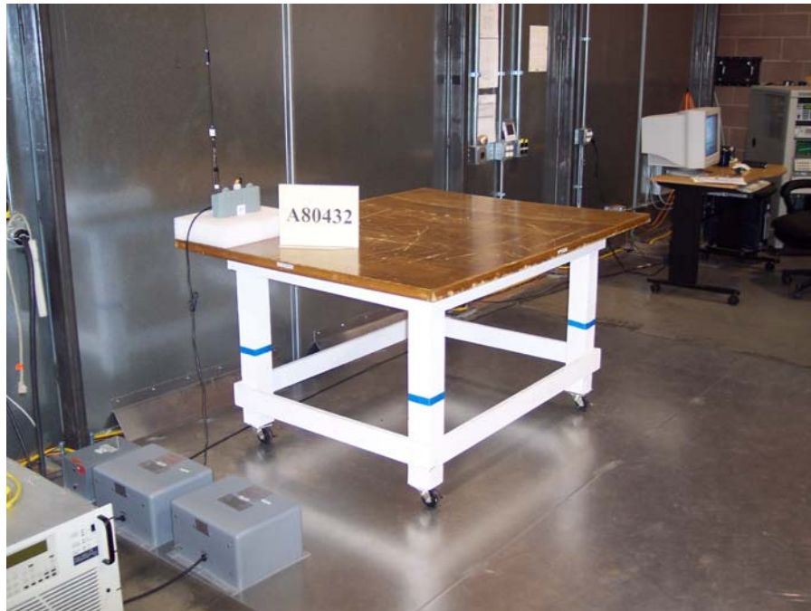
Figure 1. Representative Test Setup – Conducted Emissions, AC Mains.
