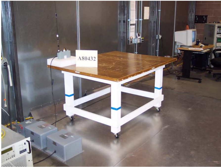
Figure 6-1. Representative Test Setup – Conducted Emissions, AC Mains.
