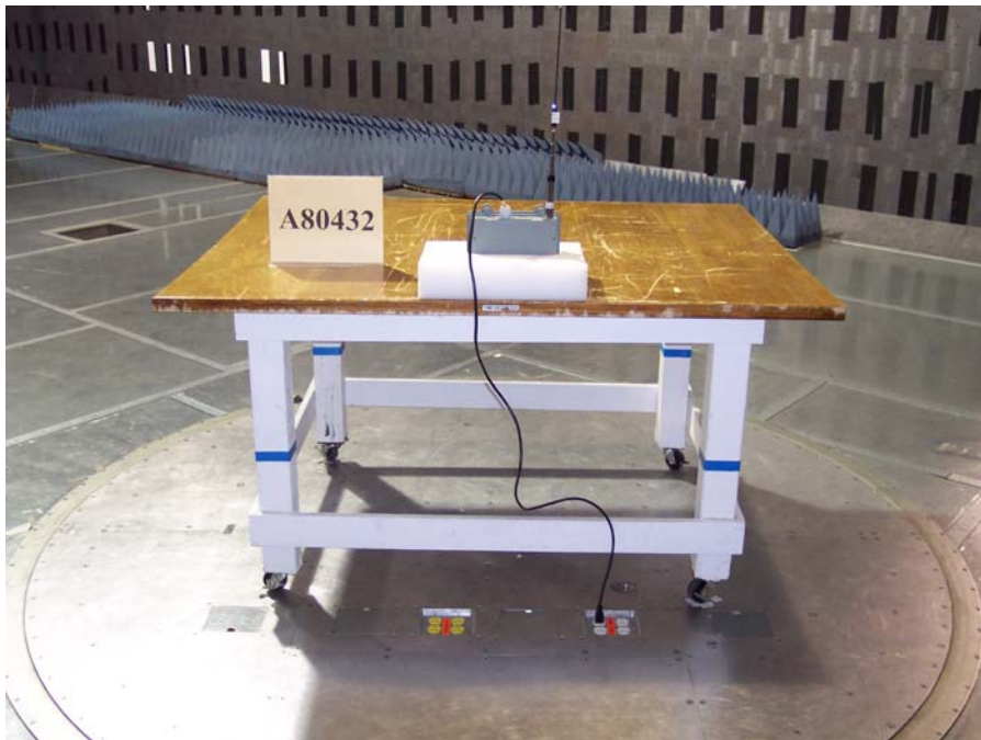
Figure 6-2. Representative Test Setup – Radiated Emissions.
