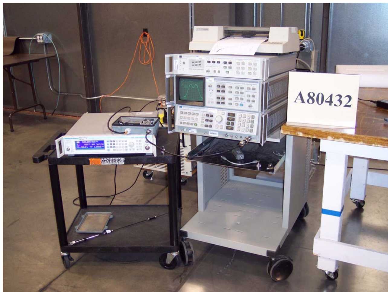
Figure F4. Test Setup, Power Spectral Density Measurement.
