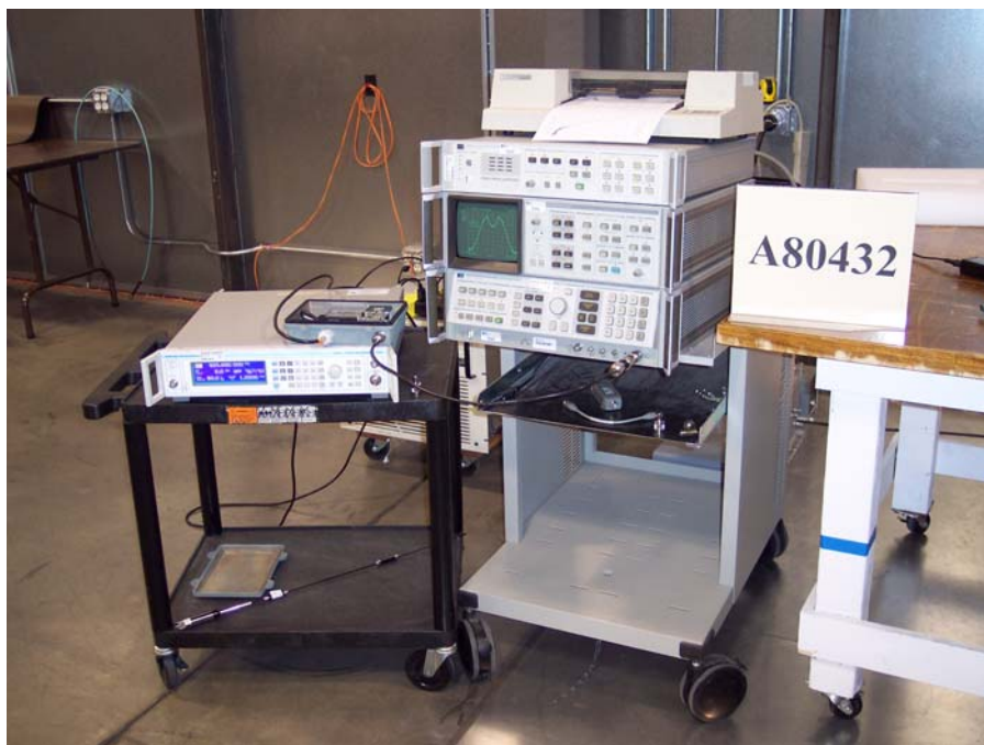
Figure 6-3. Representative Test Setup – Conducted Emissions, Antenna Terminals.
