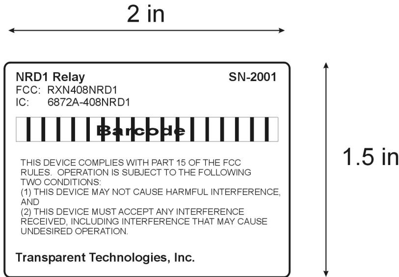
Label is permanently attached to NRD1 housing
