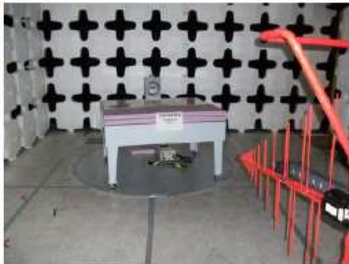
BiLog Antenna (30MHz to 1000MHz)
