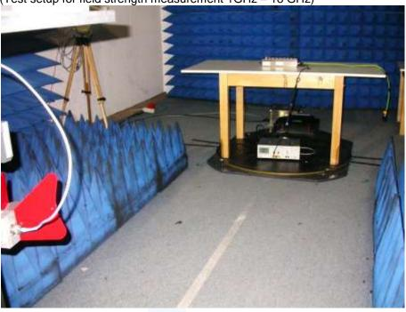
Anechoic chamber (Test setup for 18 GHz - 25 GHz)
