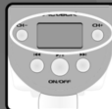
Locate the tuning buttons on your transmitter
