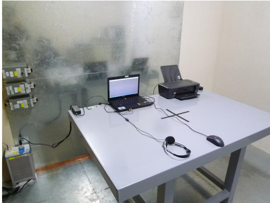
Picture 1: Conducted Emission, AC Mains; 0.15 – 30 MHz
