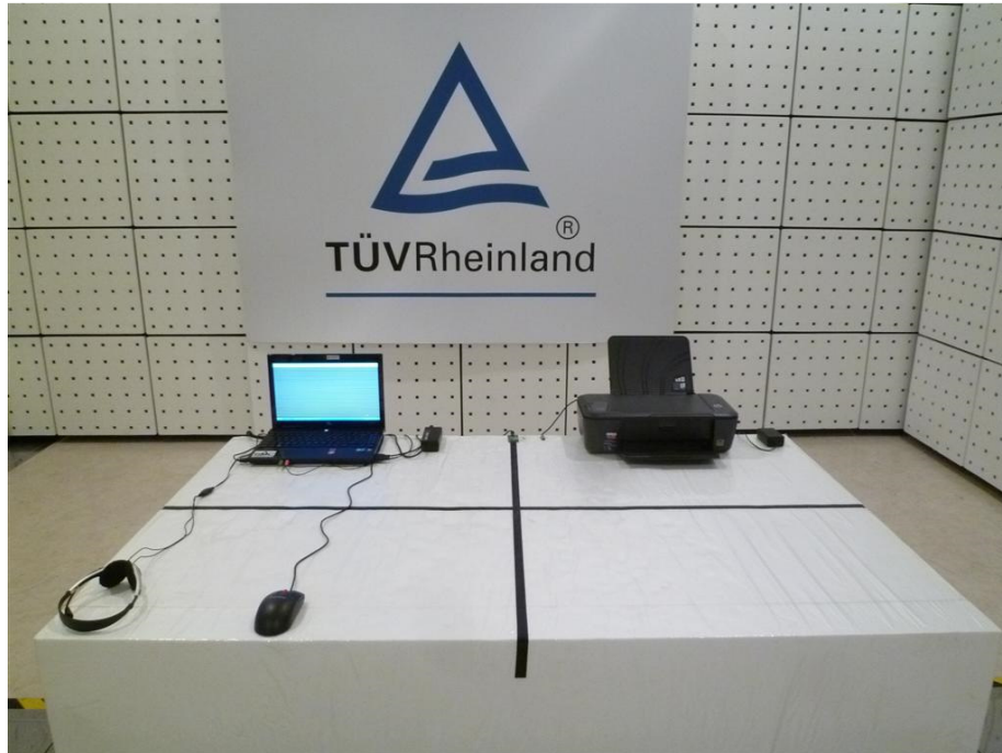
Picture 2: Radiated Emission, 30 - 1000 MHz
