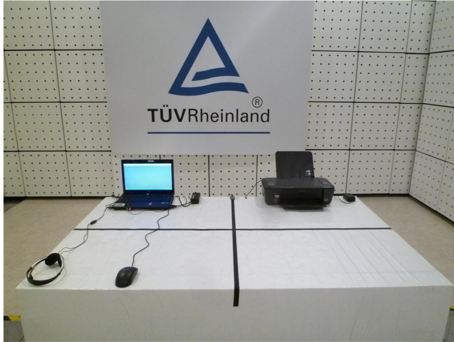
Picture 3: Radiated Emission; Above 1 GHz
