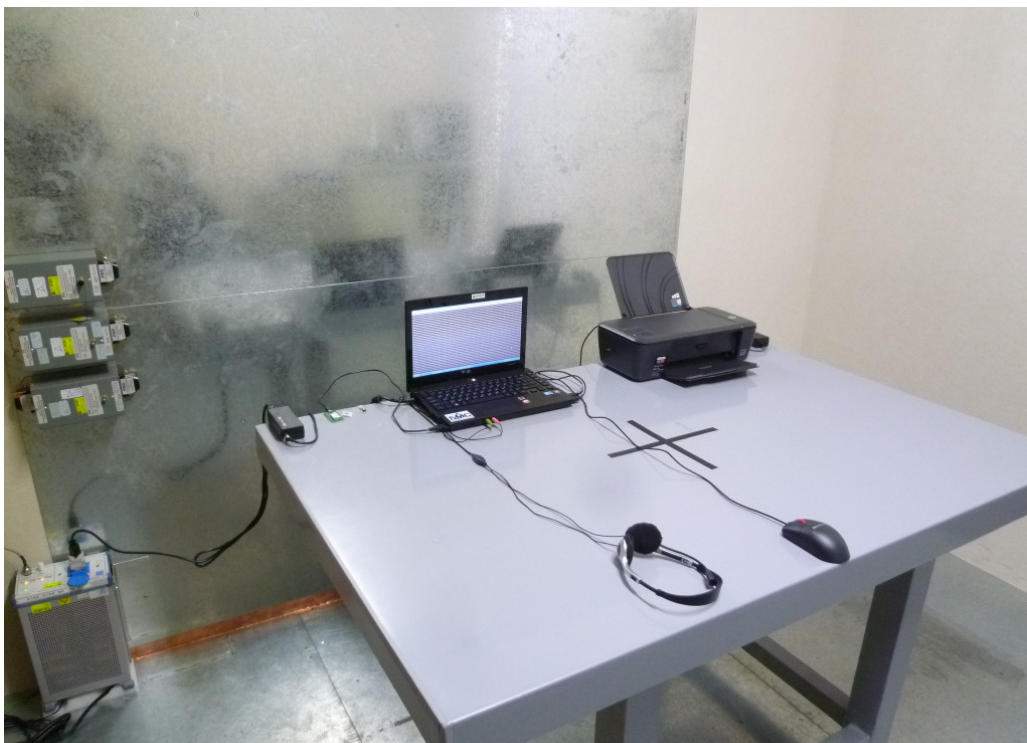
Photograph 6: Set-up for for Mains Conducted testing Front
