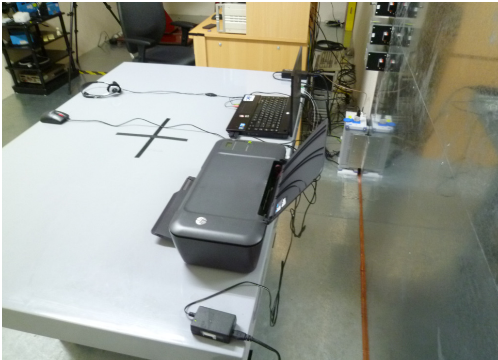
Photograph 5: Set-up for for Mains Conducted testing Back
