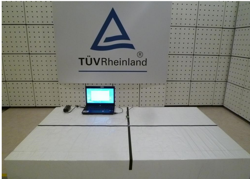
Photograph 1: Set-up for Spurious Emissions (Front View)
