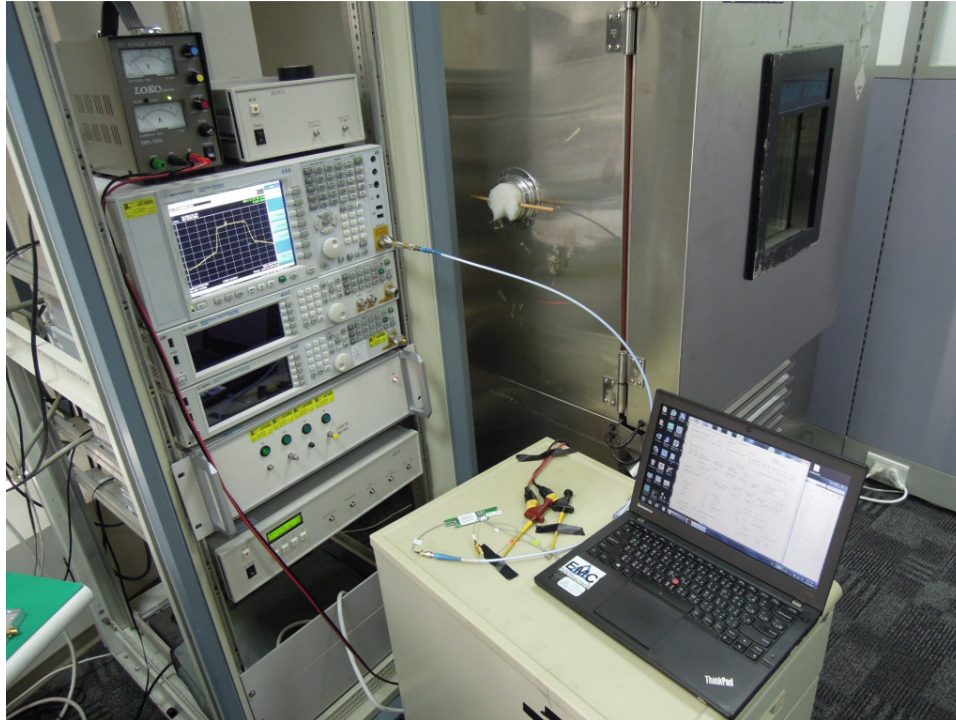
Photograph 6: Set-up for Conducted test
