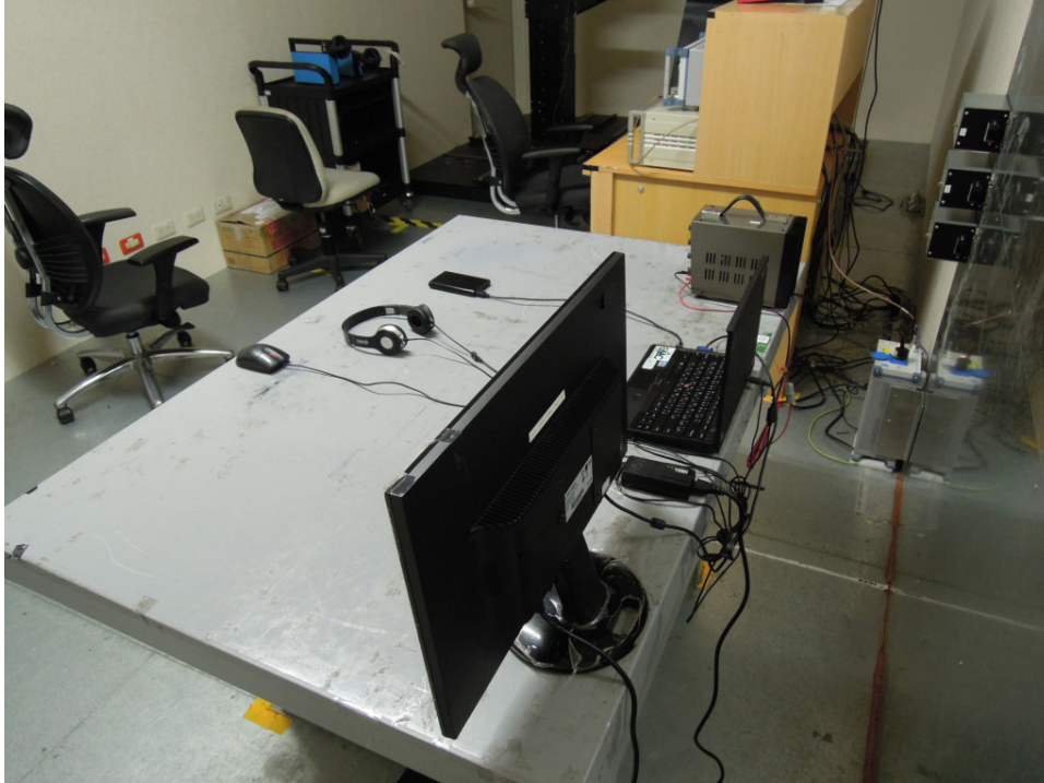
Photograph 7: Set-up for Mains Conducted testing (Back View)
