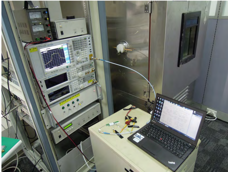
Photograph 5: Set-up for Conducted testing
