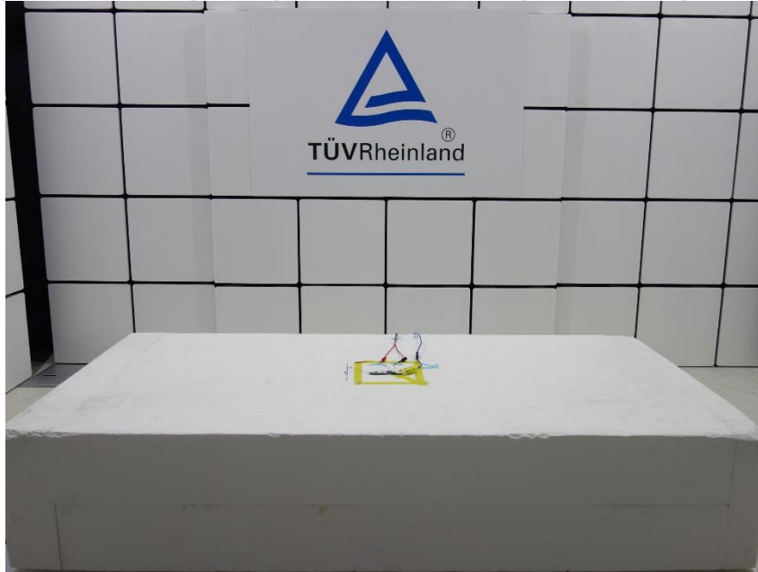
Photograph 1: Test Setup for Spurious Emissions (Front View 1)
