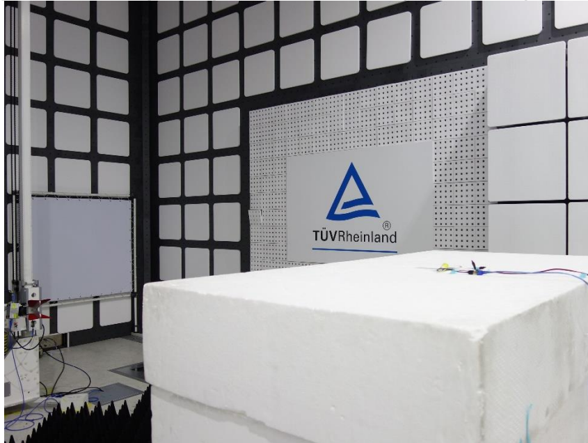
Photograph 5: Test Setup for Spurious Emissions (Back View 3)
