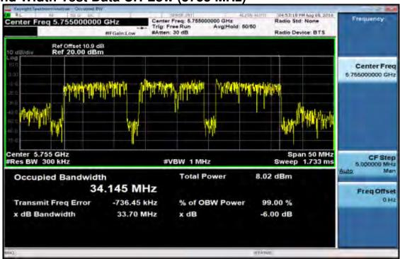
6dB Band Width Test Data CH-High (5795 MHz)
