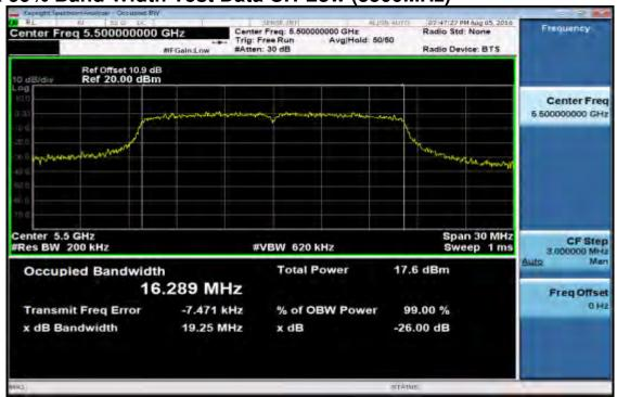
26dB & 99% Band Width Test Data CH-Mid (5580MHz)
