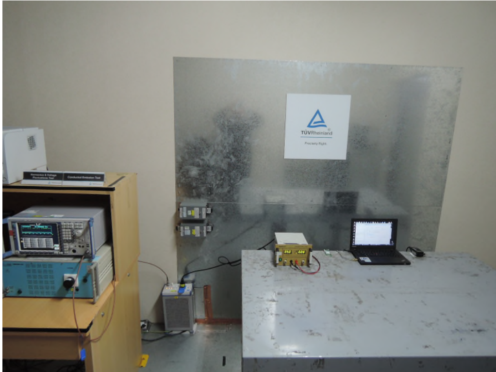
Photograph 6: Set-up for AC Mains (Back)
