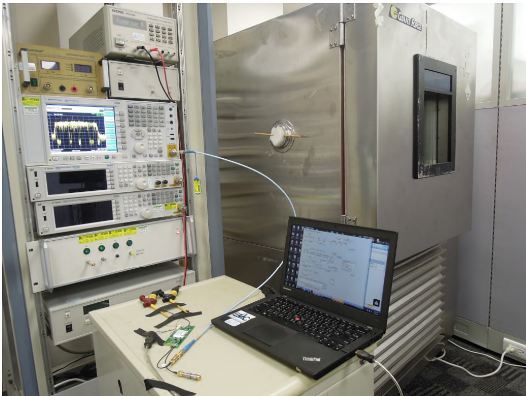
Photograph 4: Set-up for Conducted testing
