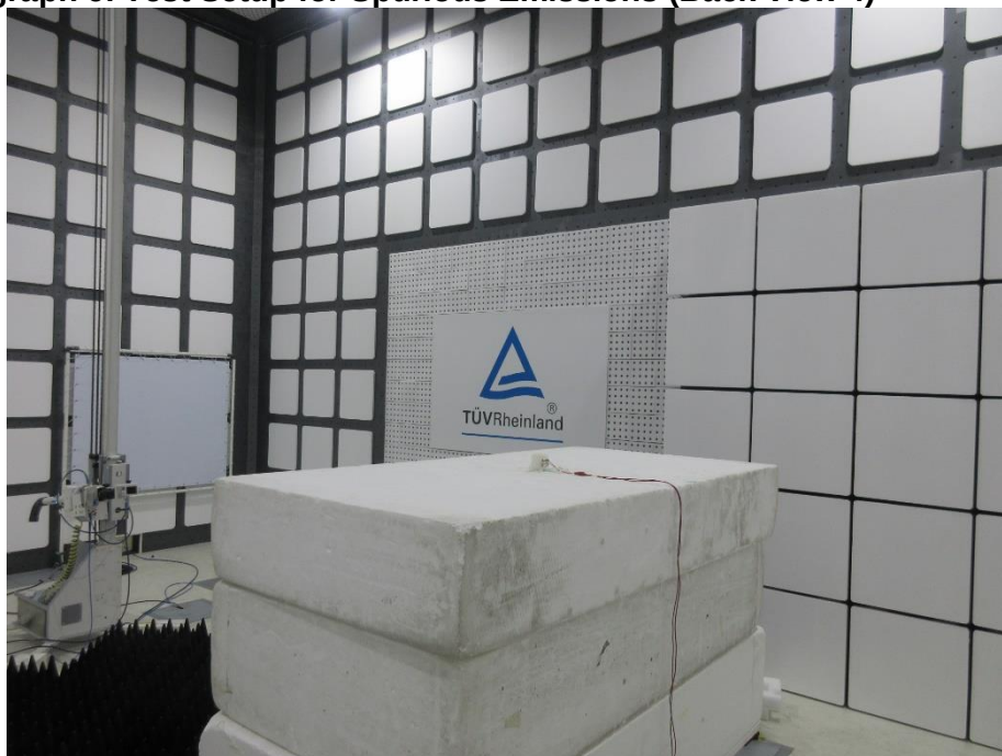
Photograph 6: Test Setup for Spurious Emissions (Back View 4)
