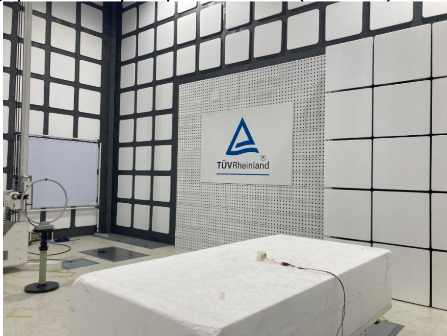
Photograph 4: Test Setup for Spurious Emissions (Back View 2)
