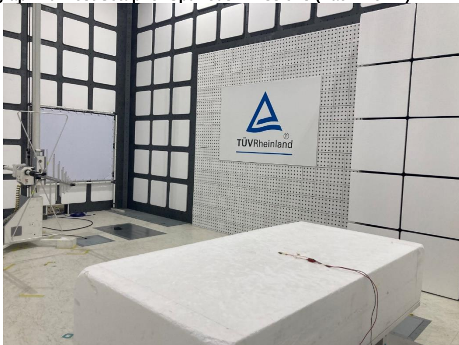
Photograph 10: Test Setup for Spurious Emissions (Back View 2)
