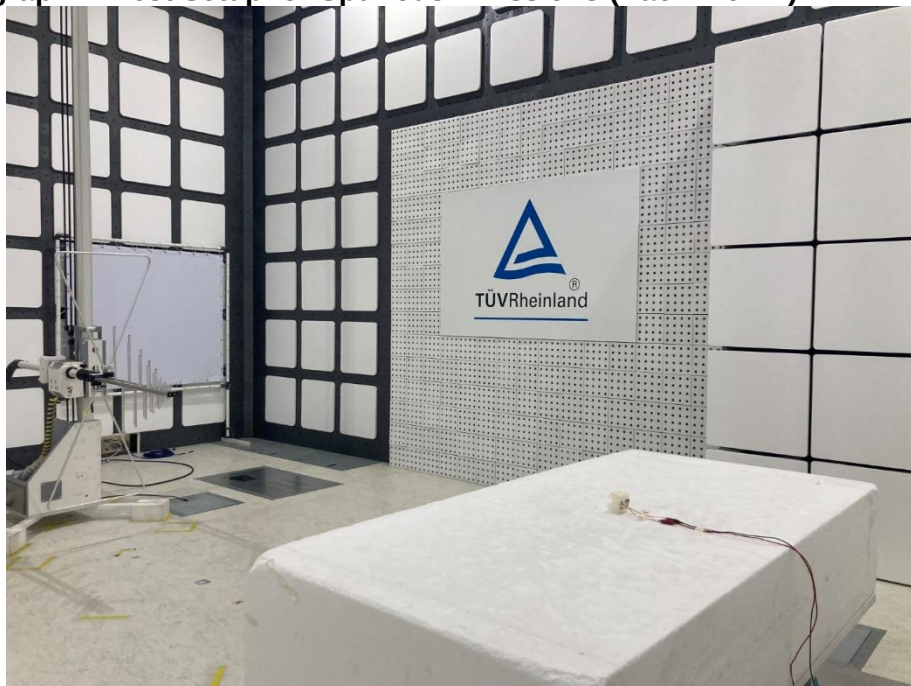
Photograph 4: Test Setup for Spurious Emissions (Back View 2)
