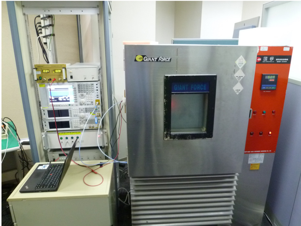
Photograph 6: Set-up for Mains Conducted testing (Back View)
