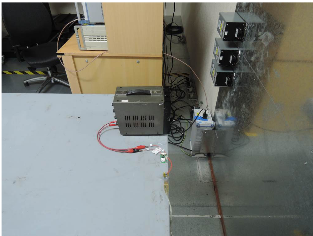
Photograph 6: Set-up for Mains Conducted testing (Back View)
