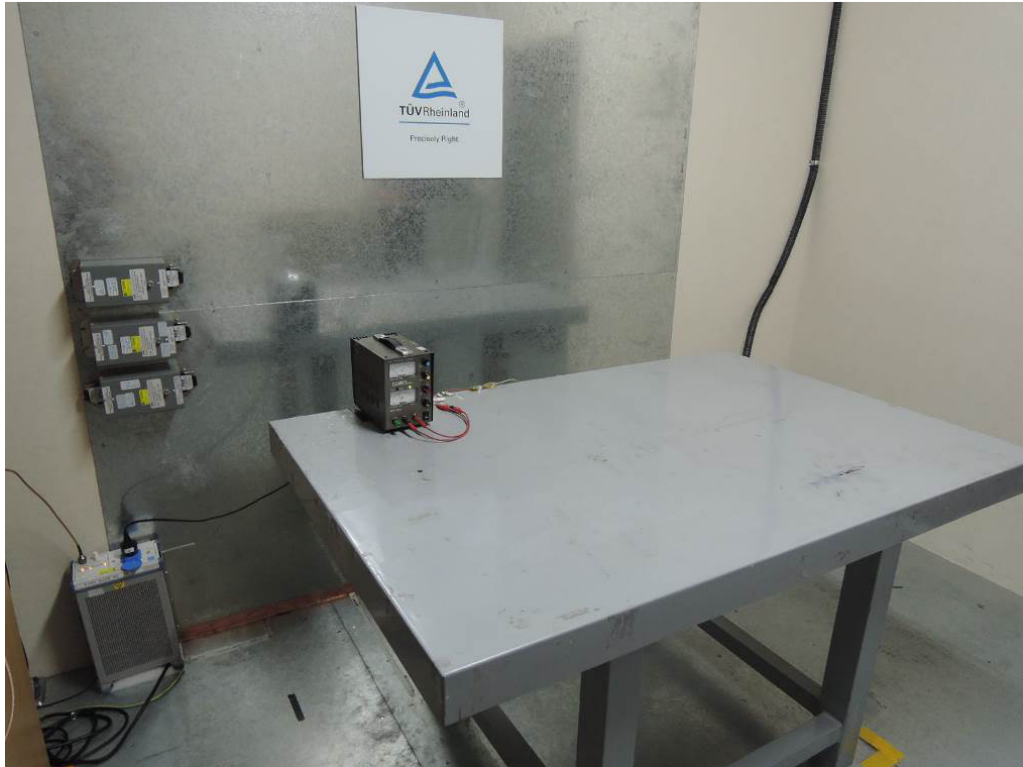
Photograph 7: Set-up for Mains Conducted testing (Front View)
