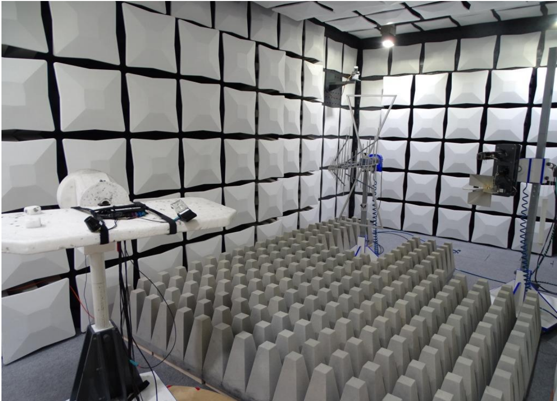
Photo 3: Test setup for radiated measurements above 1 GHz
