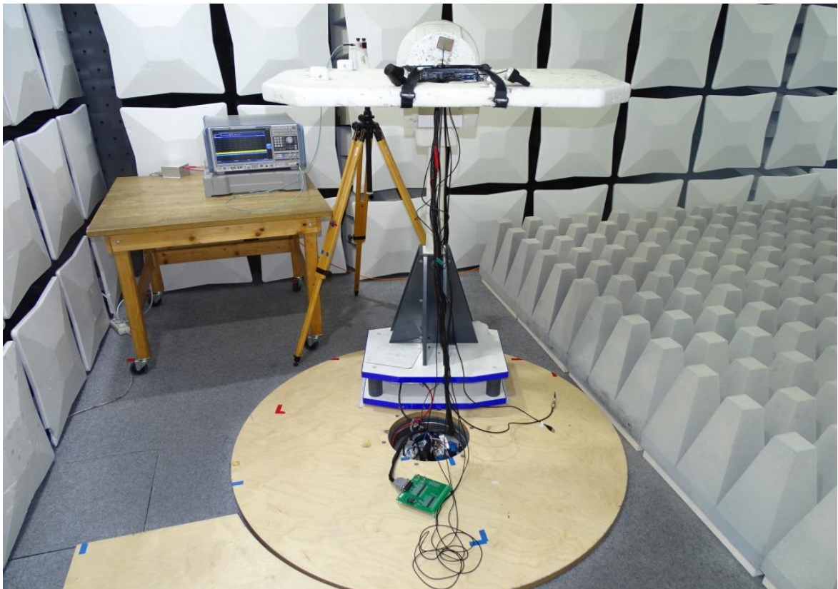
Photo 4: Test setup for radiated measurements above 26 GHz
