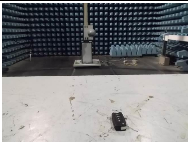
PHOTO N°3 SETUP FOR RADIATED MEASUREMENT >1GHz
