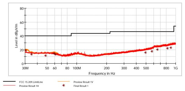
Graphic of automatic measurement from 30 MHz to 1 GHz
